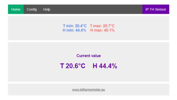
Here, you can view real-time temperature and humidity values, along with the corresponding minimum and maximum values. The Min-Max values are reset when the device is restarted, the configuration is modified and saved, or "[reset min-max] is selected in the configuration menu. The web interface automatically refreshes at predefined intervals set in the configuration menu, default value is 5 seconds.
